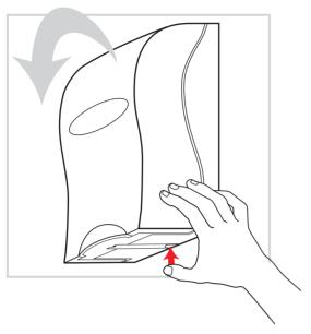
**1.** To open - press release button at the rear underside of dispenser. If necessary, ease cover forward.
