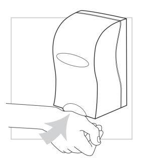
**5.** Close cover firmly and push lever several times to prime the pump.
